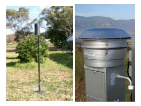
Deposited Dust and High Velocity Air Sampler.
